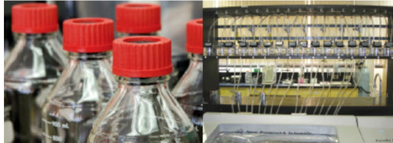
InnoTech Alberta has an automated, individual flow meter based batch culture system.
